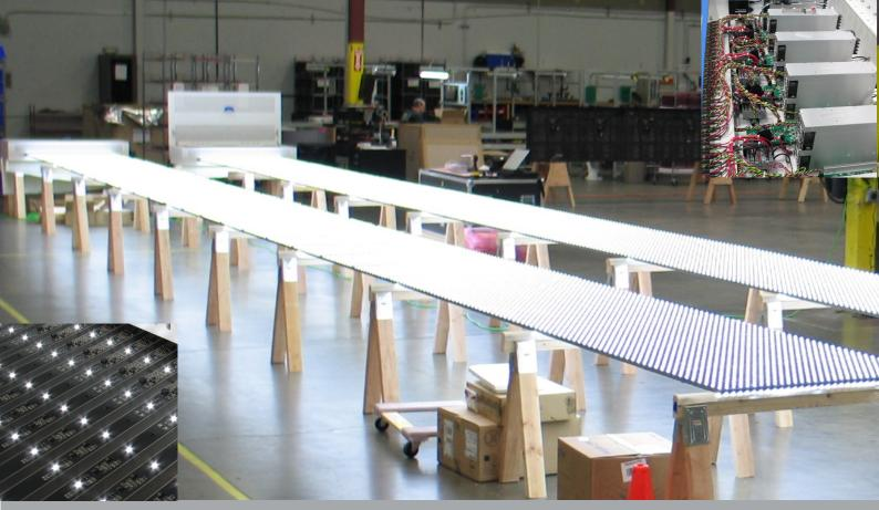
Fully suspended self supporting single & double sided transparent top mounted LED display.
